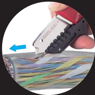
Metal guide shoe leads the cutting edge straight
